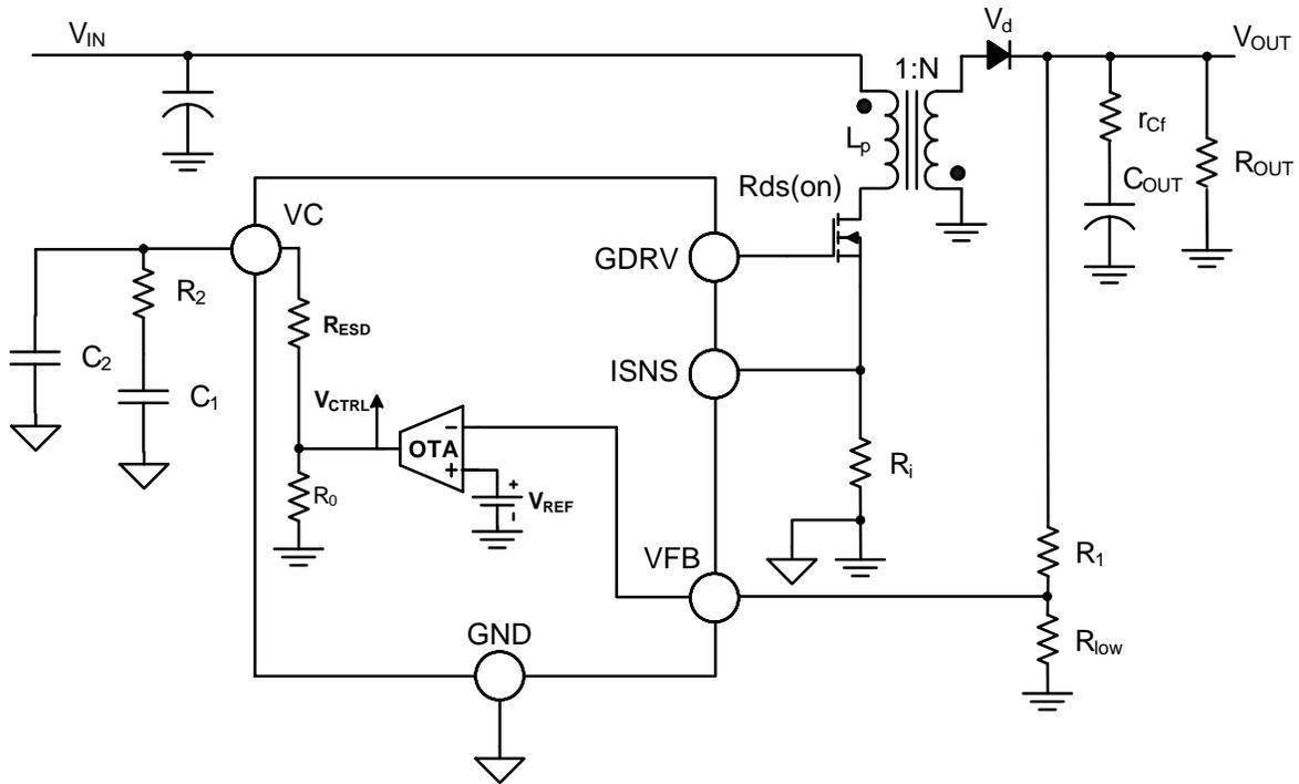
Figure 13. NCV887200 Flyback Converter OTA and Compensation
